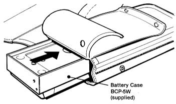
2 Place the KV-4000 on the Battery Case.
